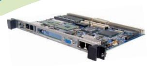
The Celero CVME-745 Intel Pentium M single-board computer is a commercial off-the-shelf (COTS) VME card used in systems that call for PC-based technology. It is designed for use in military and aerospace equipment for applications such as systems management, human interface, and processing applications.
